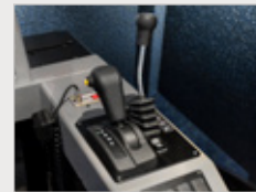
Genuine Komatsu gear selector, hoist lever, brake lock, traction, speed and brake test controls.
