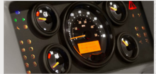
Instrument Panel integrates status indicator panels with genuine Komatsu gauge cluster to centralize all critical information.
