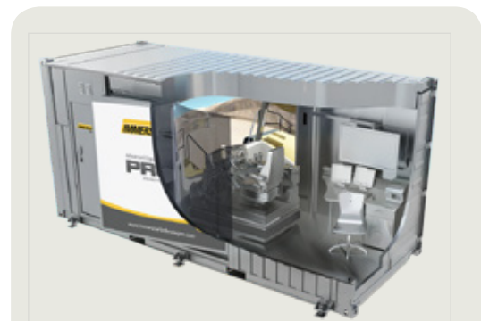
Gibraltar Mine will utilize Immersive Technologies' PRO3 Transportable Advanced Equipment Simulator for operator training
