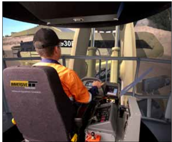
Operator using a Komatsu WA1200-3 Wheel Loader on the PRO3 simulator for surface mining
